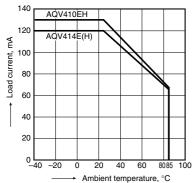
1-(2). Load current vs. ambient temperature characteristics
