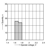
19.-(2) Operate voltage distribution Sample: AQY2C1R2P, Load voltage: 10V (DC) Continuous load current: 300mA (DC) n: 50 pcs., Ambient temperature: 25°C 77°F
