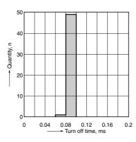
18.-(2) Turn off time distribution Sample: AQY2C1R2P, Input voltage: 5V Load voltage: 10V (DC), Continuous load current: 100mA (DC) n: 50 pcs., Ambient temperature: 25°C 77°F
