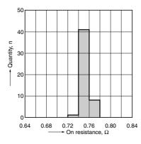
17.-(1) Turn on time distribution Sample: AQY2C1R6P, Input voltage: 5V Load voltage: 10V (DC), Continuous load current: 100mA (DC)
