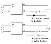
2) Even if spike voltages generated at the load are limited with a clamp diode if the circuit wires are long, spike voltages will occur by inductance. Keep wires as short as possible to minimize inductance.
