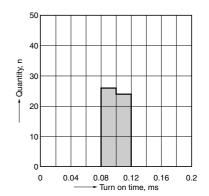
17.-(2) Turn on time distribution Sample: AQY2C1R2P, Input voltage: 5V Load voltage: 10V (DC), Continuous load current: 100mA (DC) n: 50 pcs., Ambient temperature: 25°C 77°F
