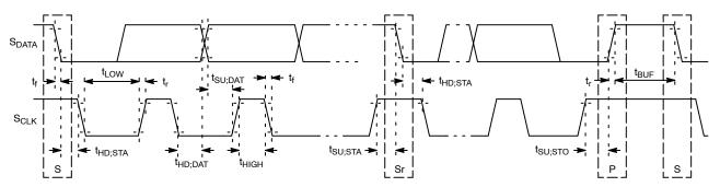
NOTE: Read sequence: For an 8-bit READ, read waveforms start after WRITE command and register address are issued.
