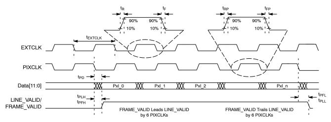
Figure 13. I/O Timing Diagram
