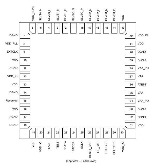
Figure 4. HiSPi 48-Lead mPLCC Package
