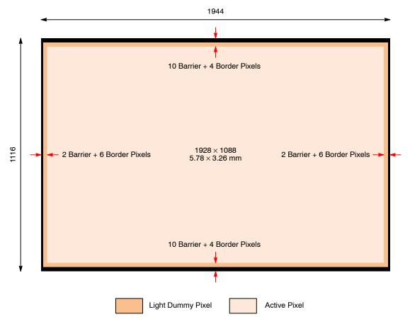
Figure 6. Pixel Array Description
