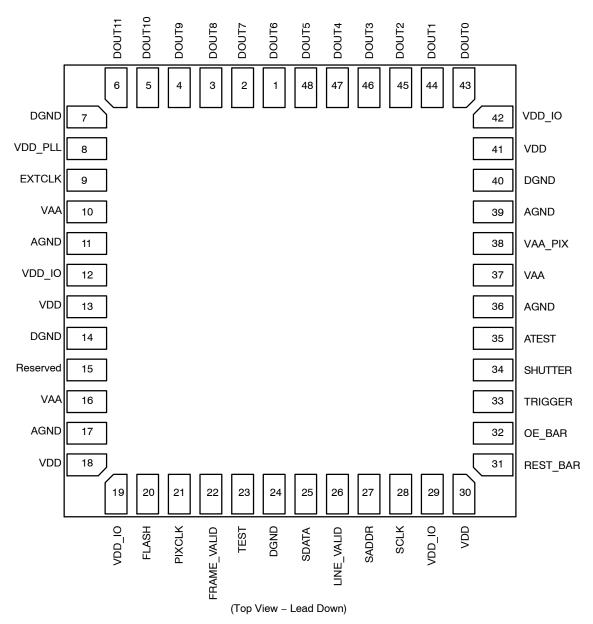
Figure 5. 48-Lead Parallel mPLCC
