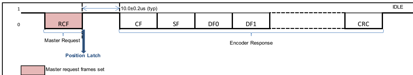
Figure 12: Encoder Data Read Out Frames Set
