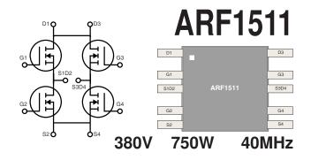
The ARF1511 is four RF power transistor arranged in an H-Bridge configuration. It is intended for off-line 300V operation in high power scientific, medical and, industrial RF power generator and amplifier applications up to 40 MHz.
