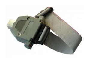
ARM debugger with JTAG and SWD interfaces, based on CoLinkEX
