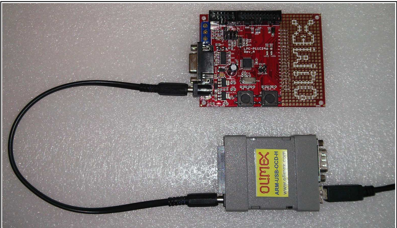
ARM-USB-OCD-H powering LPC-P11C24 (via the PWR_OUT jack).
