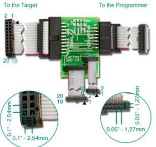
ChipProg-ISP BH14/BH20 and BH10 specialized adapter for in system programming of ARM microcontrollers .
