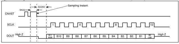
Figure 20. Single Conversion - AIN2 vs. GND (AS1525), Bipolar Mode AIN+ vs. AIN- (AS1524)
