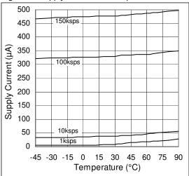
Figure 10. Supply Current vs. Sampling Rate
