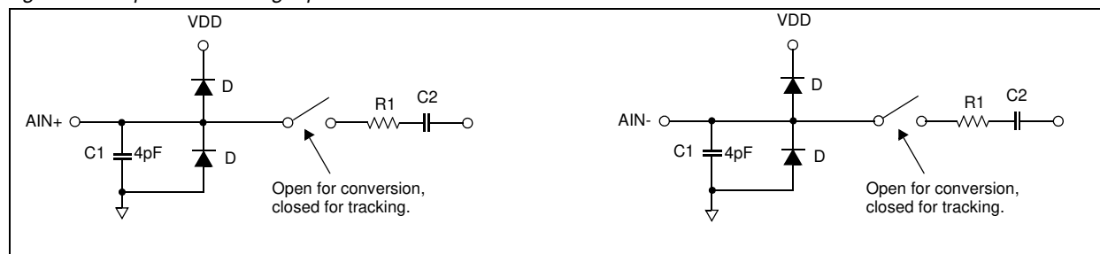
Figure 35. Equivalent Analog Input Circuit
