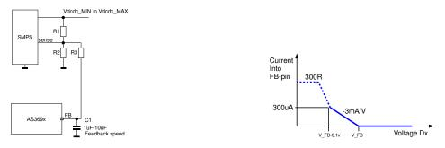
The characteristic of the feedback function can be seen in the diagram. The final output voltage of is determined by the setting of VFB and the current that is drawn from the external voltage divider.
