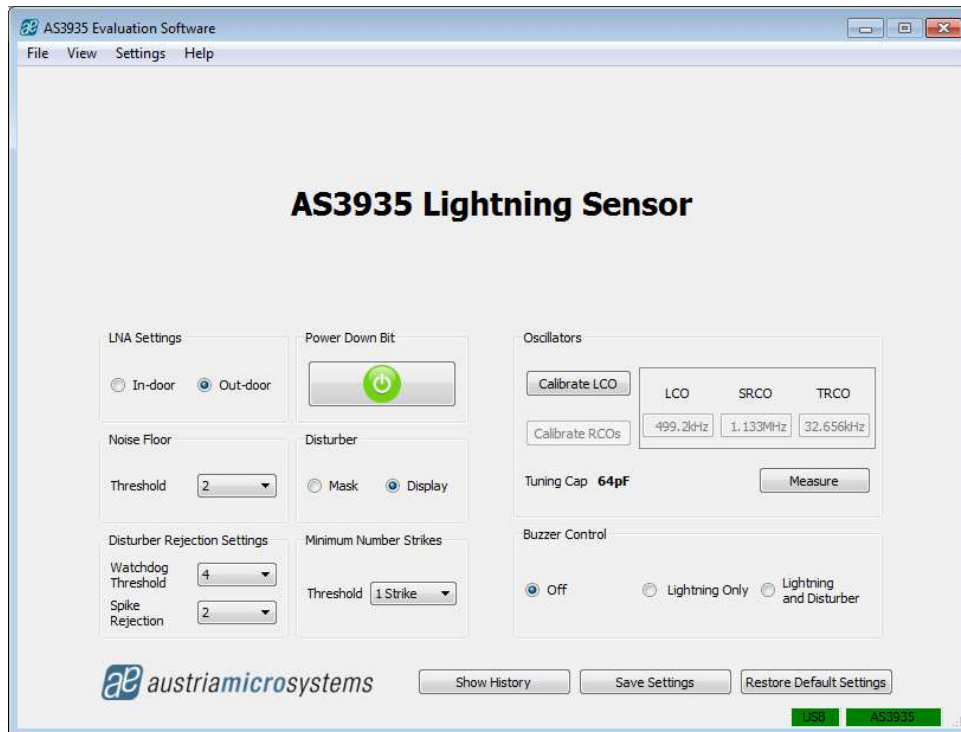
Figure 4: GUI of the AS3935 Lightning Sensor
