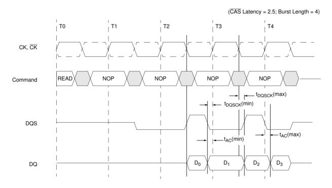
The minimum time during which the output data (DQ) is valid is critical for the receiving device (i.e., a memory controller device). This also applies to the data strobe during the read cycle since it is tightly coupled to the output data. The minimum data output valid time  $(t_{DV})$  and minimum data strobe valid time  $(t_{DQSV})$  are derived from the minimum clock high/low time minus a margin for variation in data access and hold time due to DLL jitter and power supply noise.
