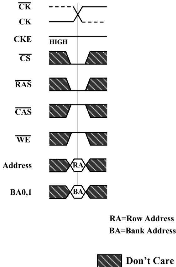
**Figure 6. t<sub>RCD</sub> and t<sub>RRD</sub> Definition**
