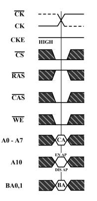
CA=Column Address BA=Bank Address EN AP=Enable Autoprecharge DIS AP=Disable Autoprecharge
