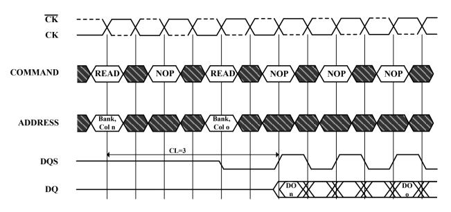
DO n (or o)=Data Out from column n (or column o) Burst Length=4 or 8 (if 4, the bursts are concatenated; if 8, the second burst interrupts the first) 3 subsequent elements of Data Out appear in the programmed order following DO n 3 (or 7) subsequent elements of Data Out appear in the programmed order following DO o Read commands shown must be to the same device
