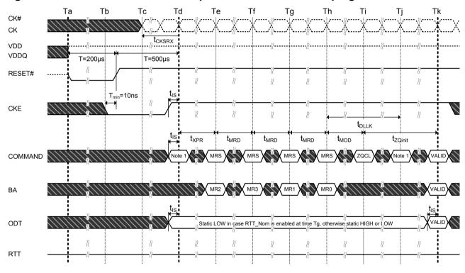
Figure 4. Reset and Initialization Sequence at Power-on Ramping
