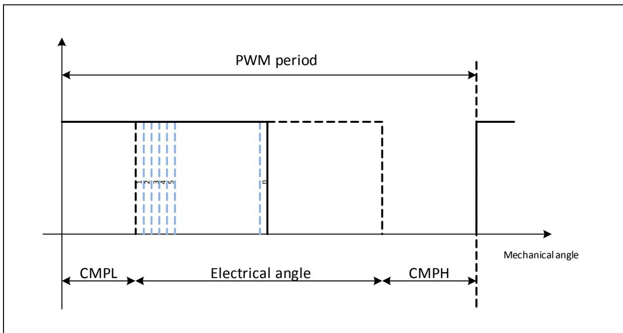
The [PWMFR](#) setting sets the duration of the PWM frequency.
