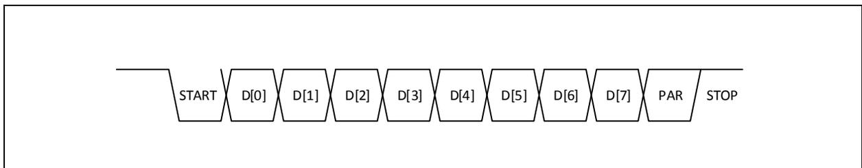
The PAR bit is even parity calculated over the data bits (D[0:7]). Each frame is transferred from LSB to MSB.
