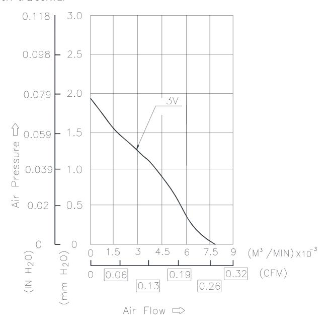
\*TEST CONDITION: INPUT VOLTAGE-----OPERATION VOLTAGE
