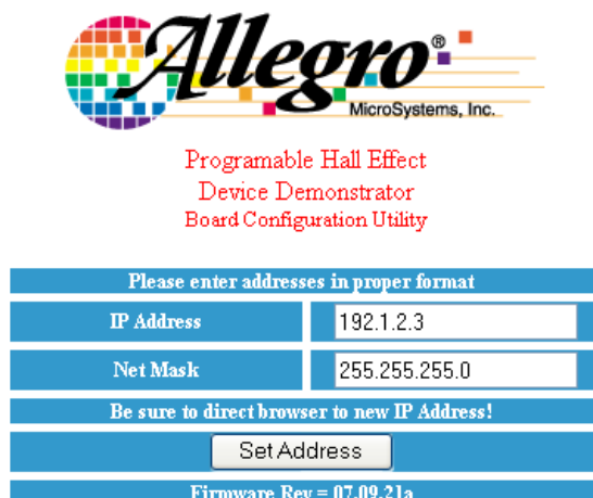
Figure 2-2 ASEK software interface, IP address setting page
