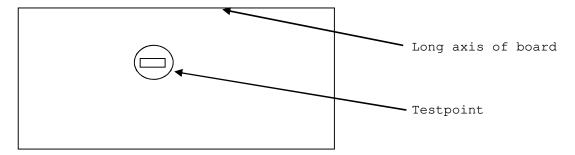
Note: loop is parallel to the long axis of the board.
