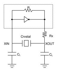
$$\begin{split} C_L &= 2^*(C_P - C_S), \\ Where \ C_P &= Load \ capacitance \ of \ crystal \ from \ crystal \ vendor \ data sheet. \\ C_S &= Stray \ capacitance \ due \ to \ C_{IN,} \ PCB, \ Trace, \ etc. \end{split}$$
