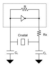
$$\begin{split} C_\text{L} &= 2^*(C_P - C_S), \\ \text{Where } C_P &= \text{Load capacitance of crystal} \\ C_S &= \text{Stray capacitance due to } C_\text{IN,} \text{ PCB, Trace etc.} \end{split}$$
