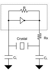
$\begin{array}{l} C_L = 2^*(C_P - C_S), \\ Where \ C_P = Load \ capacitance \ of \ crystal \\ C_S = Stray \ capacitance \ due \ to \ C_{IN,} \ PCB, \ Trace \ etc. \end{array}$
