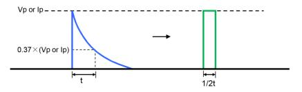
2. Damping oscillation wave with time constant of envelope "t"  $\rightarrow$  Square wave
