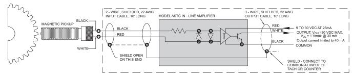
Note: Both magnetic pickup leads must be floating. Do NOT ground or connect to shield.
