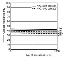
3-(2). Change in static contact resistance (10 µA 1 mV DC resistive load) Tested sample: ASX20012, 10 pcs. Operating speed: 750 cpm
