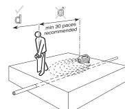
Hold the R-3000 PRO still, vertical and at right angles to the buried line. Momentarily depress the depth button. The display will show a moving clockface followed by the depth measurement.
