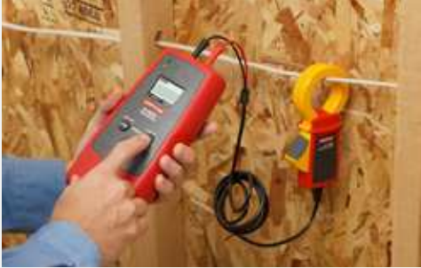
Induce signal with the signal clamp when there is no bare conductor.
