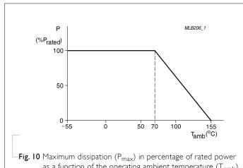
as a function of the operating ambient temperature (T<sub>amb</sub>)
