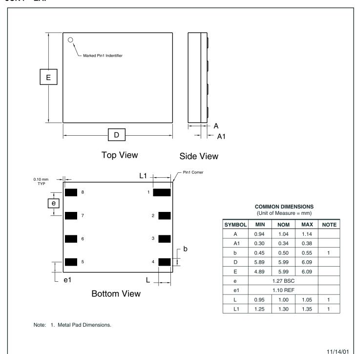
**8CN4**, 8-lead (6 x 6 x 1.04 mm Body), Lead Pitch 1.27 mm, Leadless Array Package (LAP)
