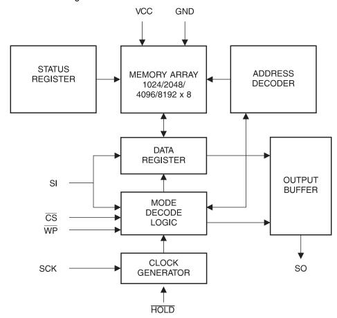
Figure 1-1. Block Diagram
