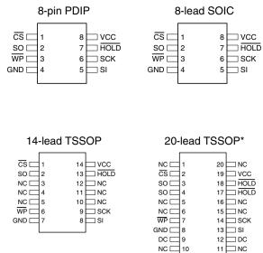
Note: \*Pins 3, 4 and 17, 18 are internally connected for 14-lead TSSOP socket compatibility.
