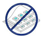
4. The outer diameter of the SMD pickup nozzle should not exceed the size of the LED to prevent air leaks. The inner diameter of the nozzle should be as large as possible.
