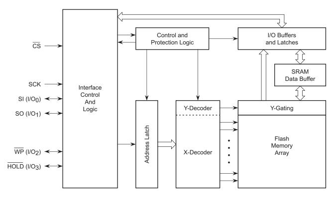
Note: I/O<sub>3-0</sub> pin naming convention is used for Dual-I/O and Quad-I/O commands.
