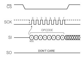
Figure 6-10. Continuous Read Mode Reset (Dual)
