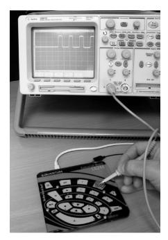
Figure 3-5. Probing X-Drive Waveforms With a Coin
