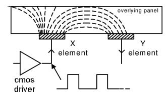
Figure 2-1. Field Flow Between X and Y Elements
