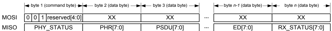
Figure 6-7. Packet Structure - Frame Read Access.
