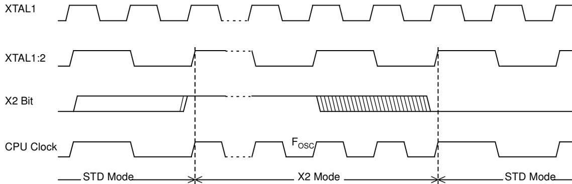
The X2 bit in the CKCON0 register (see Table 7-1) allows a switch from 12 clock periods per instruction to 6 clock periods and vice versa. At reset, the speed is set according to X2 bit of Hardware Security Byte (HSB). By default, Standard mode is active. Setting the X2 bit activates the X2 feature (X2 mode).
