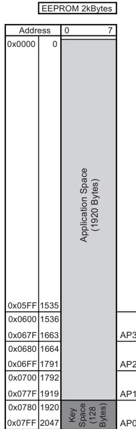
Page 2 is locked from overwriting at the end of Atmel® manufacturing. This page contains a comprehensive set of configuration and identification features. Once these have been set, they are protected from any subsequent changes.
