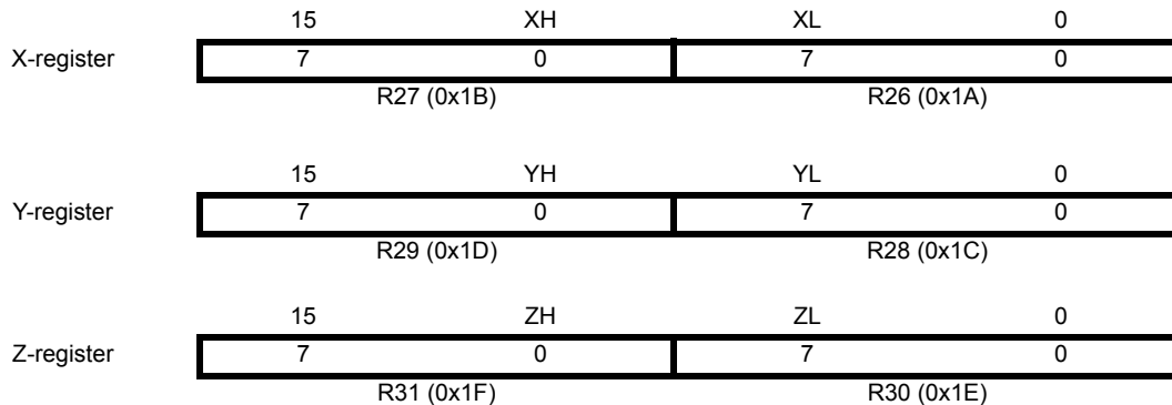
Figure 12-3. The X-, Y-, and Z-registers
