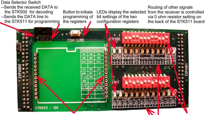
Onboard ATMega8515 uC with preset firmware controls the configuring of the register with the values selected by the DIP switches
