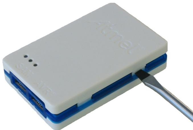
**Figure 2-14. Opening the Atmel-ICE(3)**
