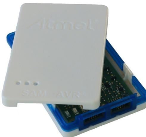
To close the unit again, simply align the top and bottom covers correctly, and press firmly together.
