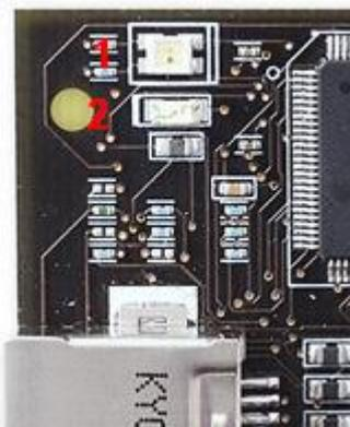
Two LEDs show the status of the Atmel AVR Dragon. Check the Troubleshooting Guide to check for solutions if there are any errors.
