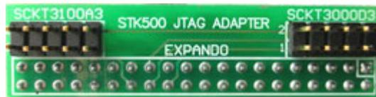
The Atmel STK500 JTAG Adapter, that is shipped with the STK500 (and previously with the JTAGICE mkII), can be used to simplify the connection to the STK500 for Atmel AVR devices with JTAG that mates with socket SCKT3100A3 and SCKT3000D3 on the STK500.
