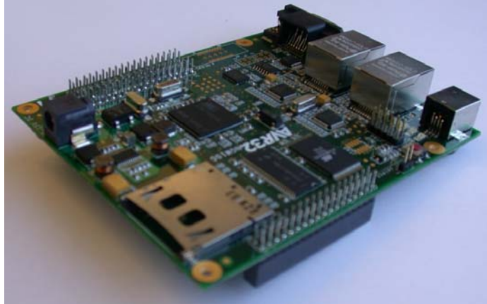
Figure 3-1. NGW100 with stack through headers inserted
