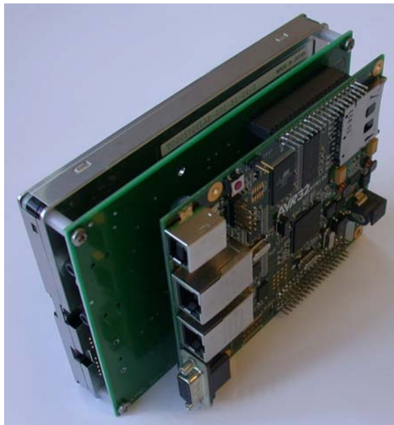
Figure 3-5. Assembled EVKLCD100 connected to a NGW100
