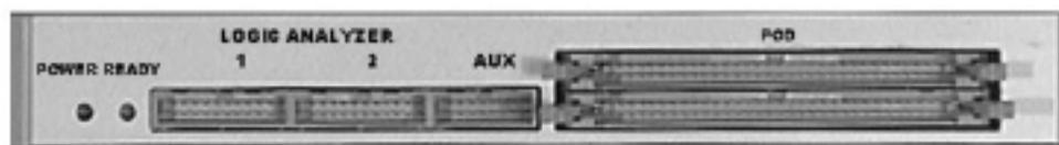
The emulator pods are connected to the **POD** connector on the ICE unit. The **LOGIC ANALYZER** and **AUX** connectors are described later. See “Connector Description” in Section 9.
