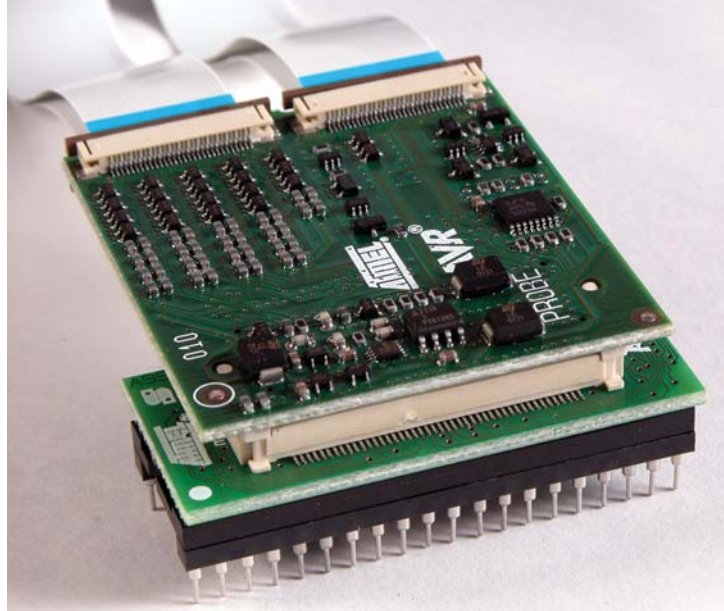
Figure 3-8. Connecting Personality Adapter to Probe
