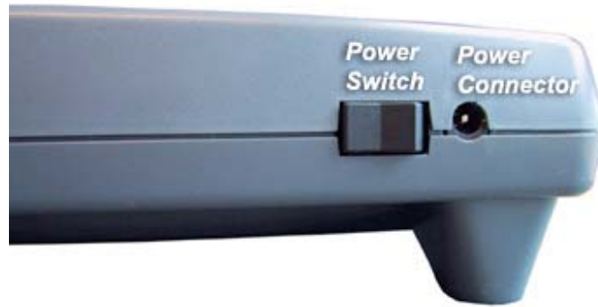
Figure 3-7. Power Switch and Connector
