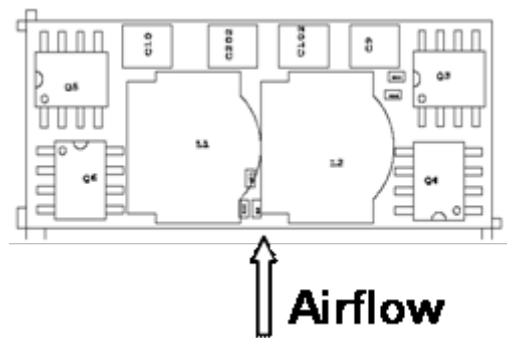
Figure 34. Airflow direction for thermal testing.
