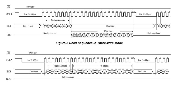
Figure-6 Write Sequence in Three-Wire Mode
