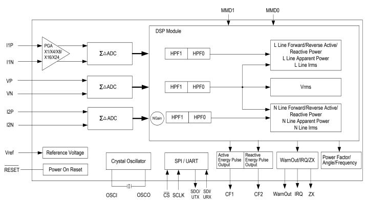
Figure-1 M90E26 Block Diagram
