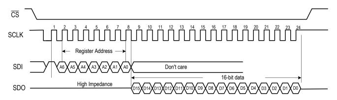
Figure-3 Read Sequence in Four-Wire Mode
