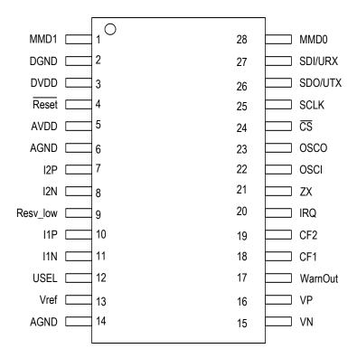
Figure-2 Pin Assignment (Top View)
