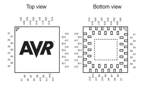
Table 1-1. DRQFN - Pinout ATmega164P/324P
