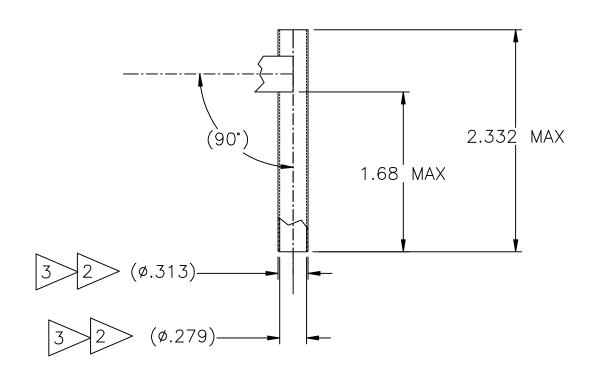
> 3. CHECK I.D. WITH GAGE PINS AND RING GAGE OVER TIP AND MINIMAL HAND PRESSURE APPLIED. 2. WITH TIPS CLOSED AROUND .274/.275¢ PIN, TIP SHALL ENTER A RING GAGE OF .317/.318 Ø. NOTES: 1. THIS IS AN AUTOCAD DRAWING DO NOT CHANGE MANUALLY
