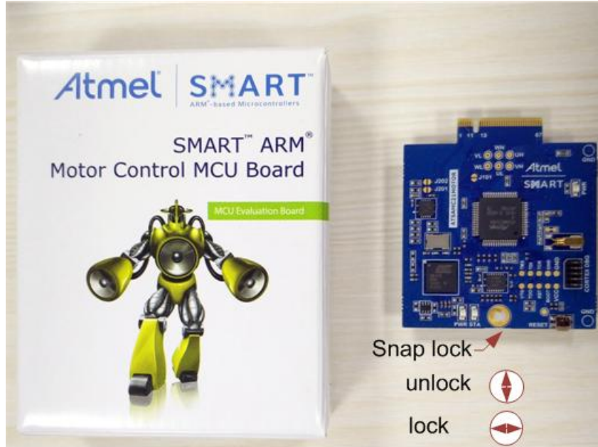
Figure 3-1. ATSAMC21MOTOR Kit Content
